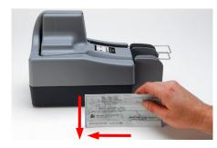
Slide the check(s) up to the line on the body of the scanner as indicated below. The left LED light will turn 'Orange'.
